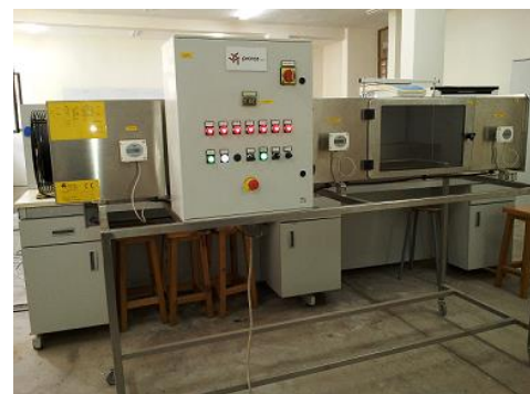
Fig.1. Tray Dryer Unit
